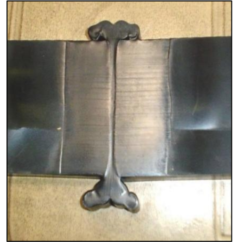
Figure 4 - Heat-Reversion Machined Pipe Wall Showing Possible Bead Shape - Left: NPS 16 DR11, Right: NPS 36 DR9
