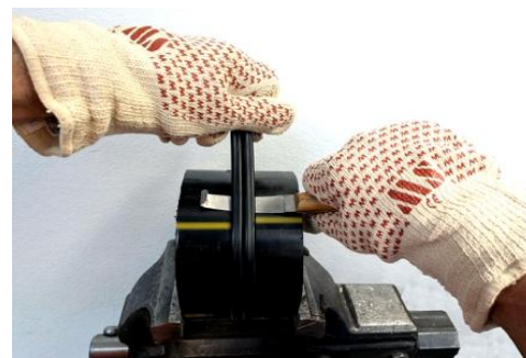
Figure 6 - Bead Removal Through Hand Skiving
