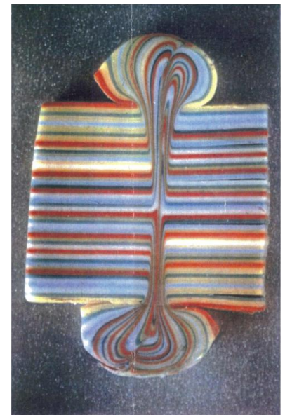
Figure 5 - Illustration of melt flow during fusion process.
