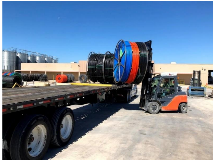
Figure 3 - Flatbed truck being unloaded on level ground.
