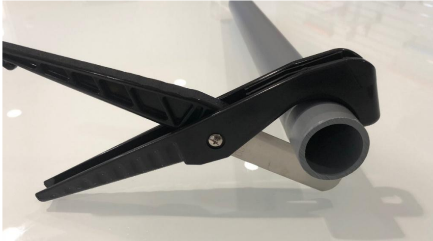
Figure 22 - Tubing cutter for smaller diameter conduit.
