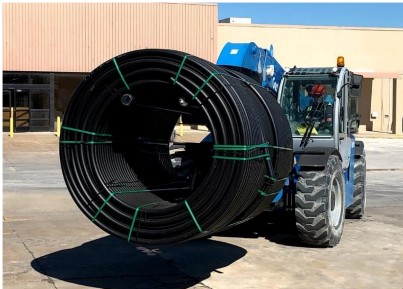
Figure 14 - Lifting a non-palletized coil through center
