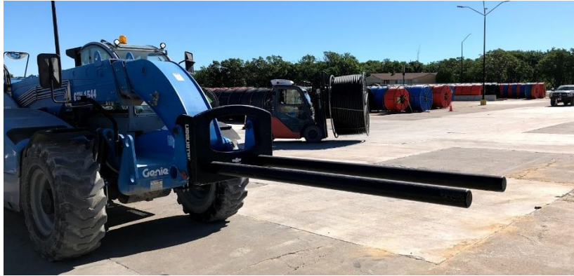
Figure 13 - Example of forklift with dual coil rams for added stability.
