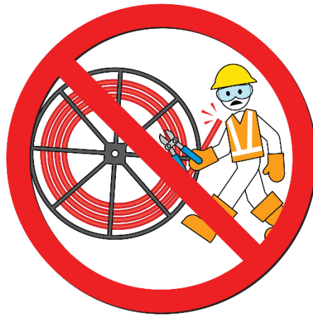
Figure 17 - Incorrectly standing in front of the coil of PE conduit while cutting, exposed to injury for rapid unwinding (spring-back) of the coil. Worker is exposed to potential for injury due to sudden spring-back of a reel of PE conduit (Images available from PPI).
