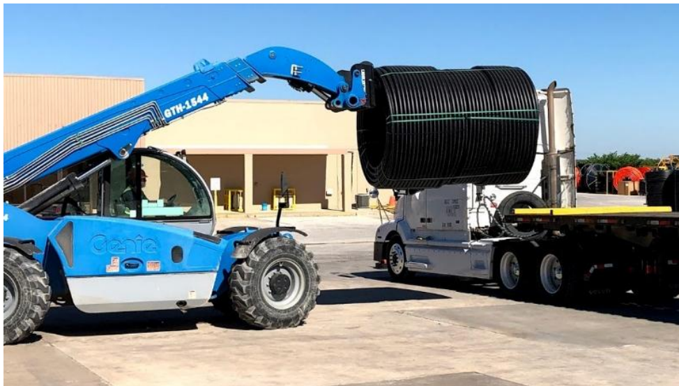
Figure 11 - Flatbed truck being unloaded on level ground – Non-palletized coils.
