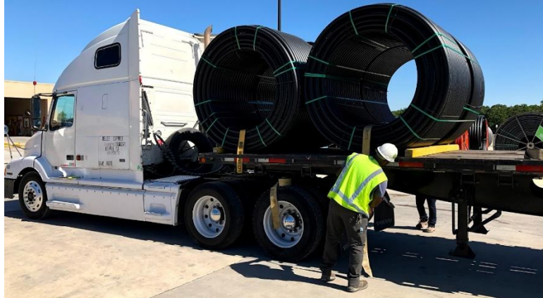
Figure 12 - Non-palletized coils chocked on trailer to prevent movement.
