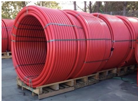
Figure 10 - Cradle palletized coils stored horizontally on level ground.
