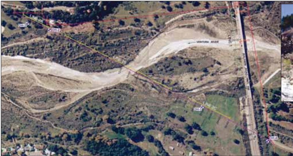
The Meiners Oaks Trunk Sewer Relocation alignment shows the existing sewer in red and new sewer in purple.
