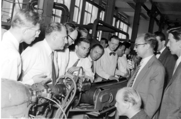
Fig. 7. Demonstration of pipe extrusion in the pilot plant of Farbwerke Hoechst, probably around the end of the 1950s
