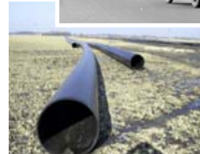
Water drainage pipes in open-cast lignite mine
