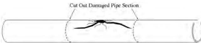
Figure 9 Cut out Damaged Section of Pipe
