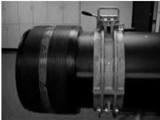
Figure 14 Hydraulic Re-Rounding Clamp Installed
