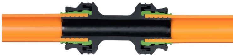
Figure 12 – Left: Cut away of an axial compression fitting design, showing application of tool to pull the compression ring over the barb thus compressing the pipe into the barbs. Right: Example of sleeve being installed with power tool (Courtesy of Viega)
