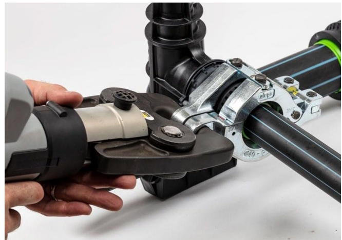
Figure 12 – Left: Cut away of an axial compression fitting design, showing application of tool to pull the compression ring over the barb thus compressing the pipe into the barbs. Right: Example of sleeve being installed with power tool (Courtesy of Viega)
