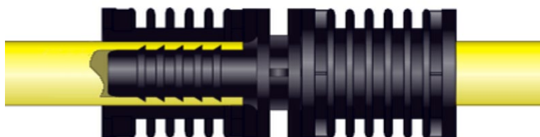
Figure 13 - Cut aways of axial compression ring fitting designs, with pipe installed (Courtesy of Viega (top), Lyall (center, bottom)).
