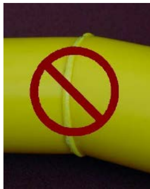
Figure A 1: Visually unacceptable mitered joint.
