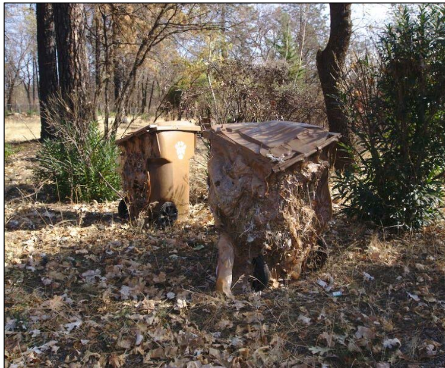
Figure 2: Yard waste bins partially melted by radiant heat from nearby house fire
