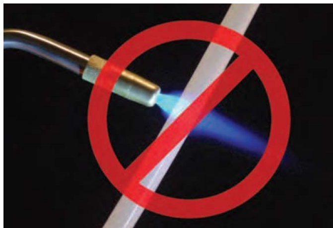
Figure 2: Do not use open flame to thaw frozen PEX pipe or tubing
